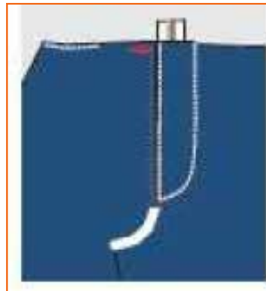
Step 17: Put a top-stitch on the edge of the finished J-piece starting from bottom to top.
