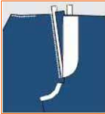
Step 14: Place the ready pattern of J-fly over the left front piece on the front rise side.
